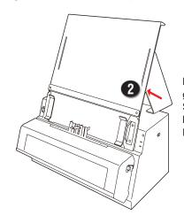
Match up the bottom groove of the Back Support with the bottom groove of the Base Tray.
