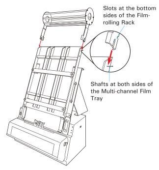
When done, fasten Quick-lock Nuts clockwise to each shaft to secure the Film-rolling Rack at the top of the Multi-channel Film Tray.
