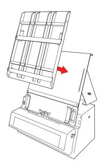
2. Pleas take note that when hooking up the Multi-channel Film Tray over the Base Tray, make sure that the hooks at the back of the Multi-channel Film Tray have been attached to the pads located at the top of the Base Tray.
